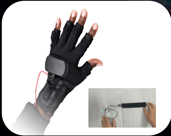
VR glove (flexible sensing+flexible battery)
